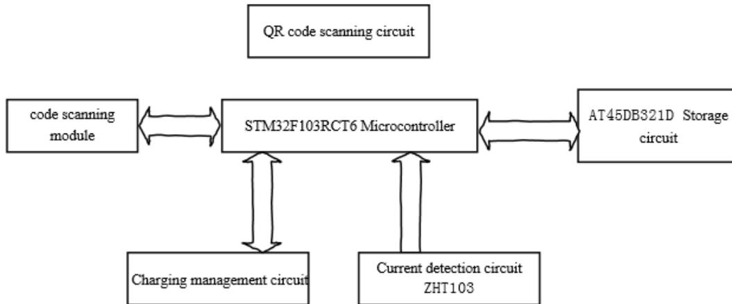
**Figure 2. Hardware overall schematic diagram.**
