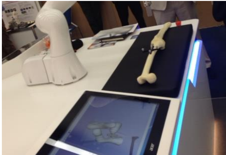
Figure 2. An example of robot-assisted interventions involves connecting Slicer to a KUKA robot to visualize 3D models of the robot, anatomy, and workspace [48, 49].
